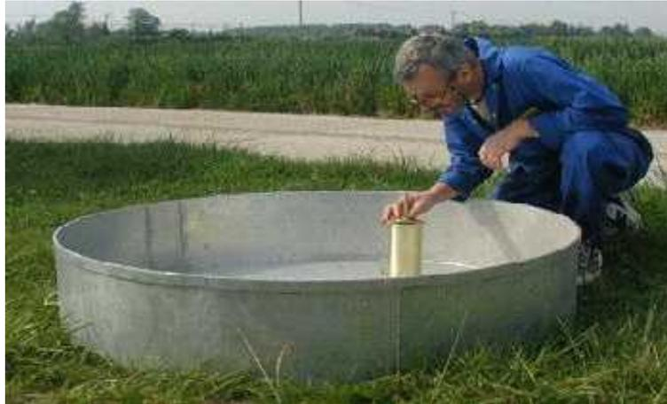
*Gambar :Open Pan Evaporimeter*
